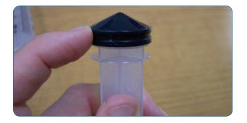
Firmly affix the rubber end to the plastic plunger by removing the rubber tip, applying glue to the "naked" end of the plunger, and replacing the rubber cap. Allow glue to cure. Then cut the conical part off the plunger tip so that only a flat surface of rubber remains.
