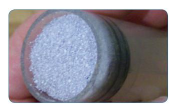
Before each sampling event, attach a fresh circular scrubbing pad to the end of the plunger. This is a head-on view of the plunger, with the scrubbing pad circle attached.
